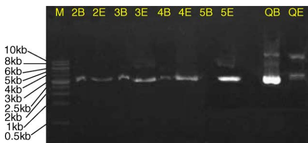
Fig. 7. Agarose electrophoresis of plasmid DNA in supernatants and elution buffer after adsorption on the PEI-modified magnetic nanobeads. Lanes: M, molecular mass marker; 2, 200 μg; 3, 300 μg; 4, 400 μg; 5, 500 μg; Q, QIAGEN; B, supernatants after adsorption; E, elution buffer.
